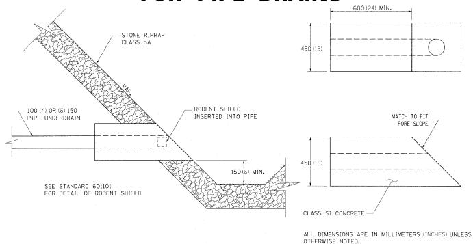
CONCRETE HEADWALLS FOR PIPE DRAINS
