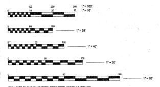
FULL SIZE PLANS HAVE BEEN PREPARED USING STANDARD ENGINEERING SCALES. REDUCED SIZED PLANS WILL NOT CONFORM TO STANDARD SCALES. IN MAKING MEASUREMENTS ON REDUCED SIZE PLANS, THE ABOVE SCALES SHALL BE USED.
