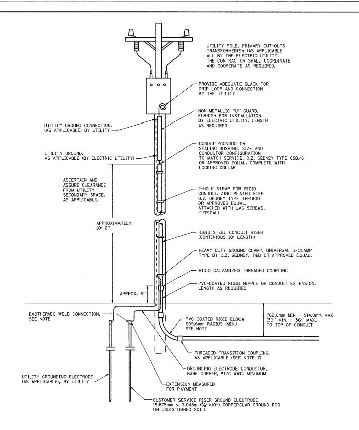
PROPOSED SERVICE INSTALLATION POLE TOP MOUNTED TRANSFORMER
