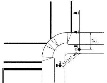
RECOMMENDED PUSHBUTTON LOCATIONS FOR ACCESSIBLE PEDESTRIAN SIGNALS SHALL BE IN ACCORDANCE WITH THE CURRENT MUTCD (SEE NOTE 1). TO MEET MUTCD REQUIREMENTS, PEDESTRIAN SIGNAL PUSHBUTTONS MAY HAVE TO BE MOUNTED ON A SEPARATE POST.
