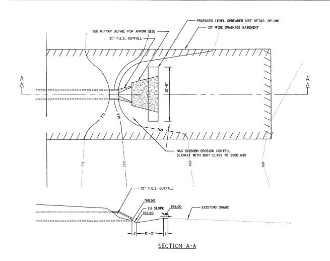
LEVEL SPREADER ALL DISTURBED AREAS TO BE RESTORED PER PLAN
