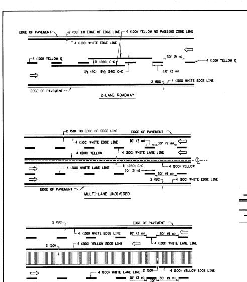
MULTI-LANE DIVIDED WITH MOUNTABLE MEDIAN NOTE: MEDIANS WITH BARRIER CURB DO NOT REQUIRE AN EDGE LINE
