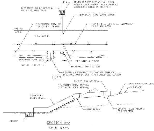
TEMPORARY SLOPE DRAIN SHALL BE USED AT THE TOP OF FILL SLOPE AS EMBANKMENT IS CONSTRUCTED TO PREVENT EXCESSIVE EROSION UNTIL SHOULDERS ARE CONSTRUCTED AND THE SLOPES ARE SEEDED AND MULCHED.
