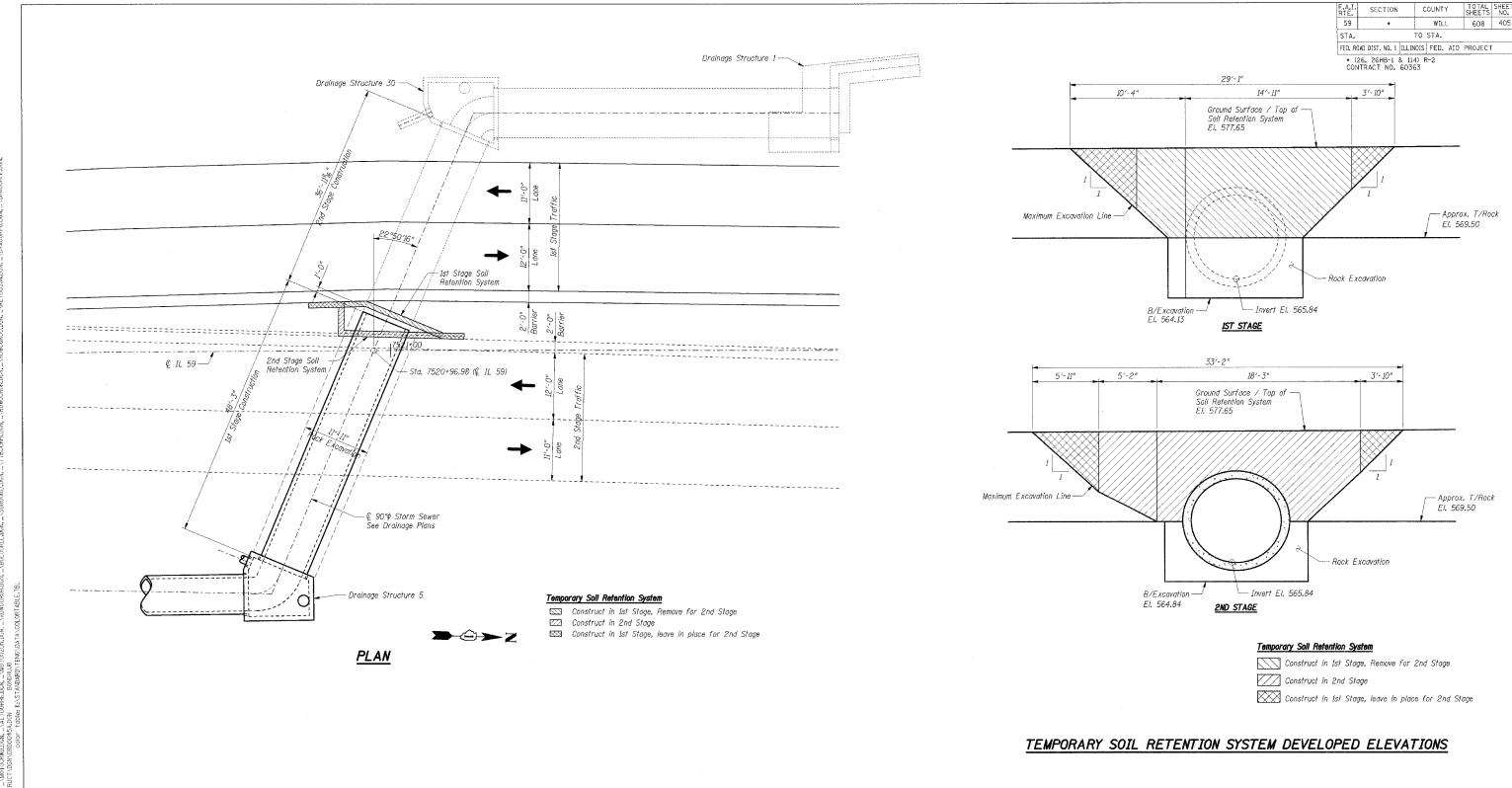
A cantilevered sheet piling design does not appear feasible and additional members or other retention systems may be necessary. The Contractor shall submit a temporary soil retention system design including plan details and calculations for review and acceptance by the Engineer.
