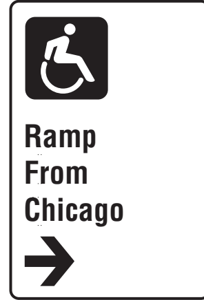
Sign Type 7.14 Used to direct disabled commuters to ramp to trains coming from Chicago.
