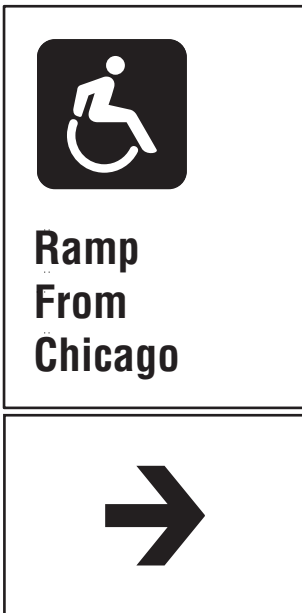
Sign Type 4.8 Used to direct disabled commuters to ramp to trains that are coming from Chicago.
