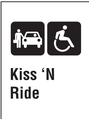
Sign Type 4.3a Used to identify accessible Kiss 'N Ride drop off
