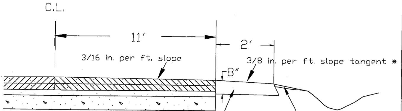
PROPOSED HOT MIX ASPHALT SHOULDER TO BE CONSTRUCTED IN TWO LIFTS AS DIRECTED BY THE ENGINEER. BOTH LIFTS TO BE HOT MIX ASPHALT SURFACE MIX C.
