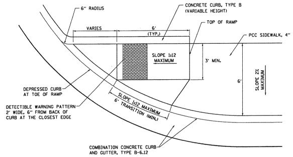
NOTE: SEE PLANS FOR LOCATIONS. FOR SIDEWALK RAMP AT STA. 101+62 RT ON BRIDGE APPROACH PAVEMENT, REFER TO BRIDGE PLANS SHEET 28 OF 55 FOR CONSTRUCTION DETAILS.
