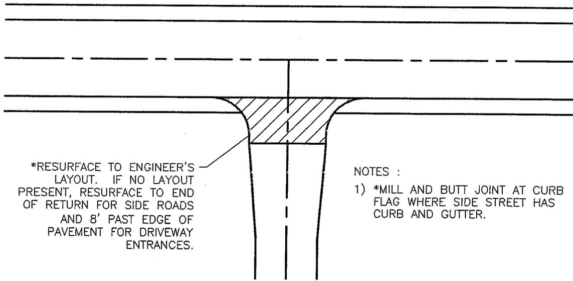
\*RESURFACE TO ENGINEER'S LAYOUT. IF NO LAYOUT PRESENT, RESURFACE TO END OF RETURN FOR SIDE ROADS AND 8' PAST EDGE OF PAVEMENT FOR DRIVEWAY ENTRANCES.
