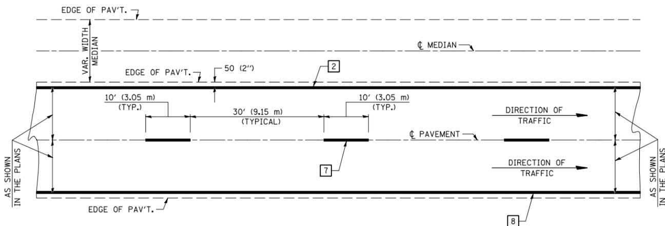
NOTE: PAVEMENT MARKINGS ARE TO BE EXTENDED THROUGH OMISSIONS WHEN APPLICABLE.
