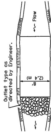
The long dimension should be parallel with the direction of the flow. Accumulated silt shall be removed anytime the basins become 75% filled.
