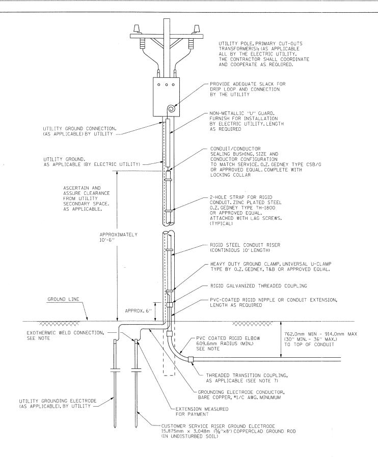
PROPOSED SERVICE INSTALLATION POLE TOP MOUNTED TRANSFORMER
