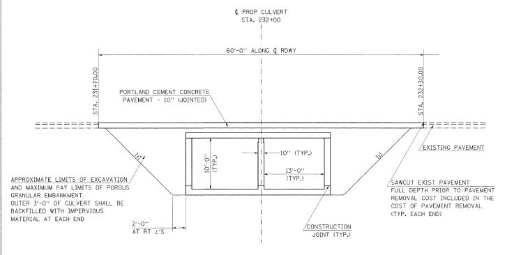
NOTE: POROUS GRANULAR EMBANKMENT WILL BE CA7 OR CA11 WITH THE TOP 1' CONSISTING OF CA6 OR CA10.
