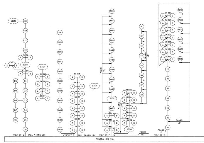
\*6AWG UD=UNIT DUCT, 600V, 2-1C NO.6, 1/C NO.6 GROUND, (XLP-TYPE USE), 1" DIA. POLYETHYLENE AND ELECTRIC CABLE IN CONDUIT, 600V (XLP-TYPE USE) 3-1/C NO. 6
