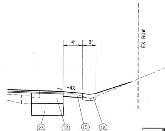
**PROPOSED GUTTER SECTION - LEFT OR RIGHT**
