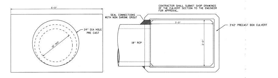
18" RCP TO 3"X2" PRECAST BOX CULVERT CONNECTION
