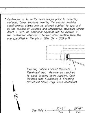
© Transverse tie £'s (3 per span). Place additional shims at midpoints between tie &'s. Securely weld shims to top flange of support beam. Minimum shim size is 6" x flange width.
