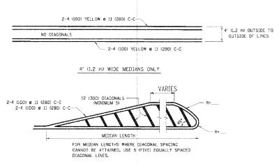
DIAGONAL LINE SPACING: 50' (15 m) C-C (LESS THAN 30MPH (50 km/h)) TEY (25 m) C-C 30MPH (50 km/h) TO 45MPH (70 km/h)) 150' (45 m) C-C (MORE THAN 45MPH (70 km/h))
