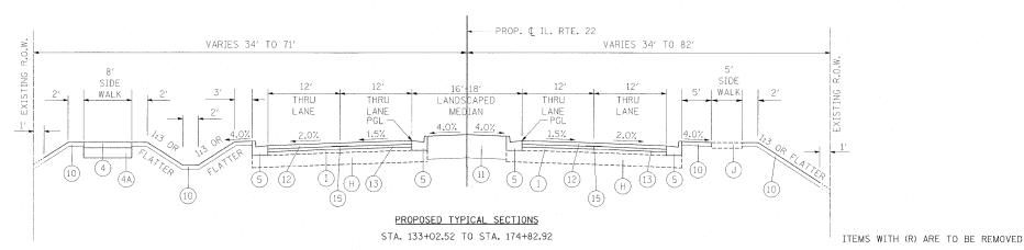
\*\*MOUNTABLE CURB AND GUTTER TO BE USED FROM APPROXIMATELY STA. 97+90 TO STA. 98+73
