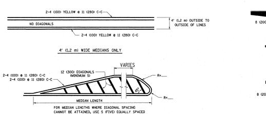
DIAGONAL LINE SPACING: 50' (15 m) C-C (LESS THAN 30MPH (50 km/h))
