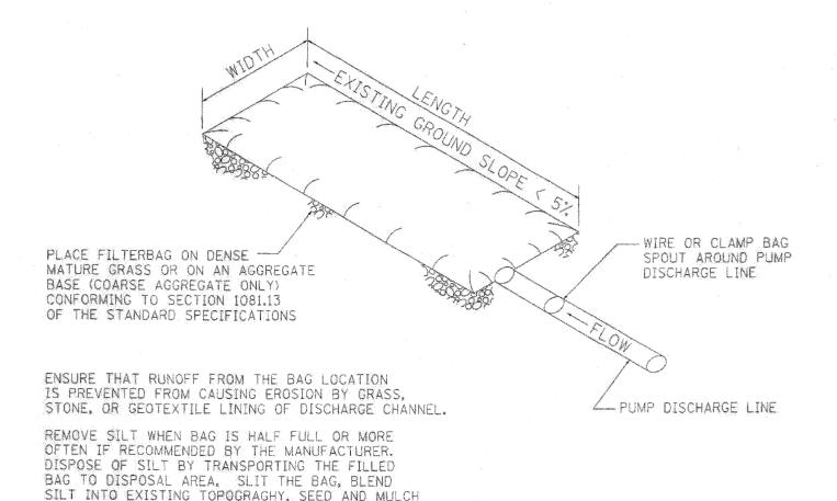
FIGURE S1. SEDIMENT FILTER BAG
