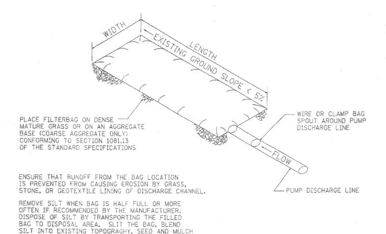
FIGURE S1. SEDIMENT FILTER BAG
