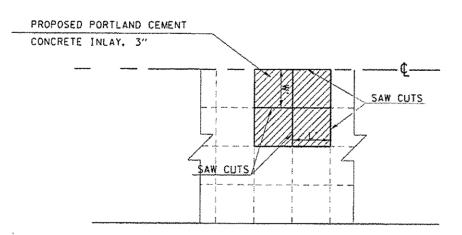
SAW CUTS SHALL BE MADE AT ALL EXISTING JOINTS FOR PAVEMENT REMOVAL (SPECIAL) AND FOR PORTLAND CEMENT CONCRETE INLAY, 3"
