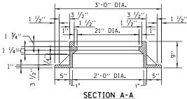
NOTE: METAL PLATES MUST BE FURNISHED FOR PERFORATED LIDS ON MANHOLES.
