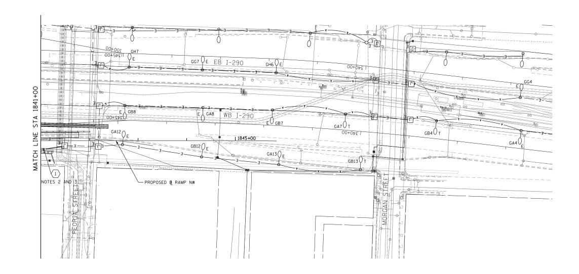
CKTS GA & GB: 3-1/C NO. 2 & 1-1/C NO. 4 GROUND XLP TYPE USE CABLES IN 1 1/2" POLYETHYLENE UNIT DUCT NOTE 4
