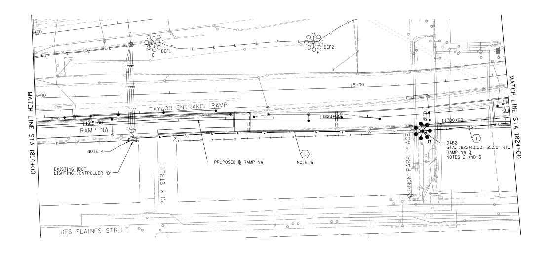
1) CKTS. DA & DB: 3-1/C NO. 2 & 1-1/C NO. 4 GROUND XLP TYPE USE CABLES IN 1 1/2" POLYETHYLENE UNIT DUCT
