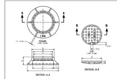
NOTES: LETTERING FOR CHICAGO W.W. ON THE LID SHALL BE 1" SHARR FACE GOTHIC LETTERS, 3/6" WIDE AND RAISED '2" FROM '2" RECESS AS MEASURED FROM THE TOP SURFACE OF THE LID.
