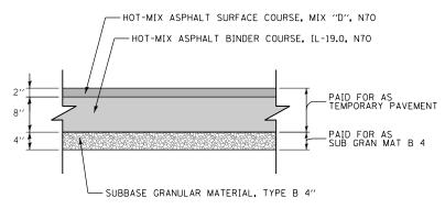
TEMPORARY HMA PAVEMENT FOR TEMPORARY RAMP NW, TEMPORARY RAMP SW, AND TAYLOR ENTRANCE RAMP
