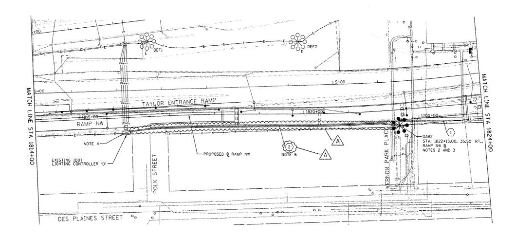
CKTS, DA & DB: 3-1/C NO. 2 & 1-1/C NO. 4 GROUND XLP TYPE USE CABLES IN 1 1/2" POLYETHYLENE UNIT DUCT
