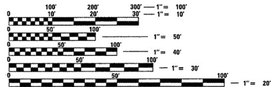
FULL SIZE PLANS HAVE BEEN PREPARED USING STANDARD ENGINEERING SCALES. REDUCED SIZED PLANS WILL NOT CONFORM TO STANDARD SCALES. IN MAKING MEASUREMENTS ON REDUCED PLANS, THE ABOVE SCALES MAY BE USED.
