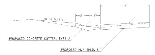
CONCRETE GUTTER, TYPE A TO BE CONSTRUCTED
