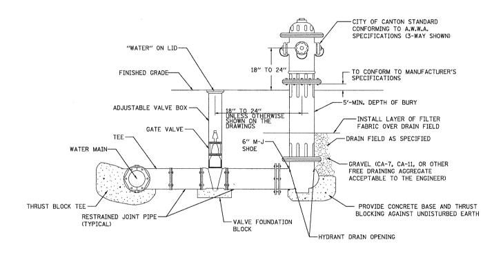
NOTE: CONCRETE BASE AND BLOCKING MATERIAL SHALL NOT BLOCK NOR OBSTRUCT HYDRANT DRAINS
