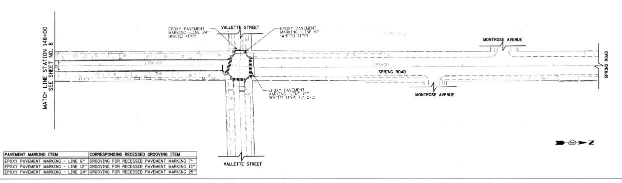
NOTES: 1) EPOXY PAVEMENT MARKINGS SHALL BE INSTALLED IN GROOVED RECESSED CHANNELS CONSTRUCTED 0.040 INCHES BELOW THE SURFACE AND 1 INCH WIDER THAN THE PAVEMENT MARKING LINE. CONSTRUCTION OF THE RECESSED CHANNELS SHALL BE PAID FOR SEPARATELY PER FOOT AS GROOVING FOR RECESSED PAVEMENT MARKING OF THE WIDTH SPECIFIED AND PER SQUARE FOOT FOR GROOVING FOR RECESSED PAVEMENT MARKING, LETTERS, NUMBERS AND SYMBOLS.
