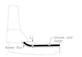
Repair of the existing deck slab shall include but may not be limited to the areas shown. The actual area to be repaired will be determined by the Engineer at the time of construction. Cost of existing joint removal is included in the cost of Silicone Joint Sealer.
