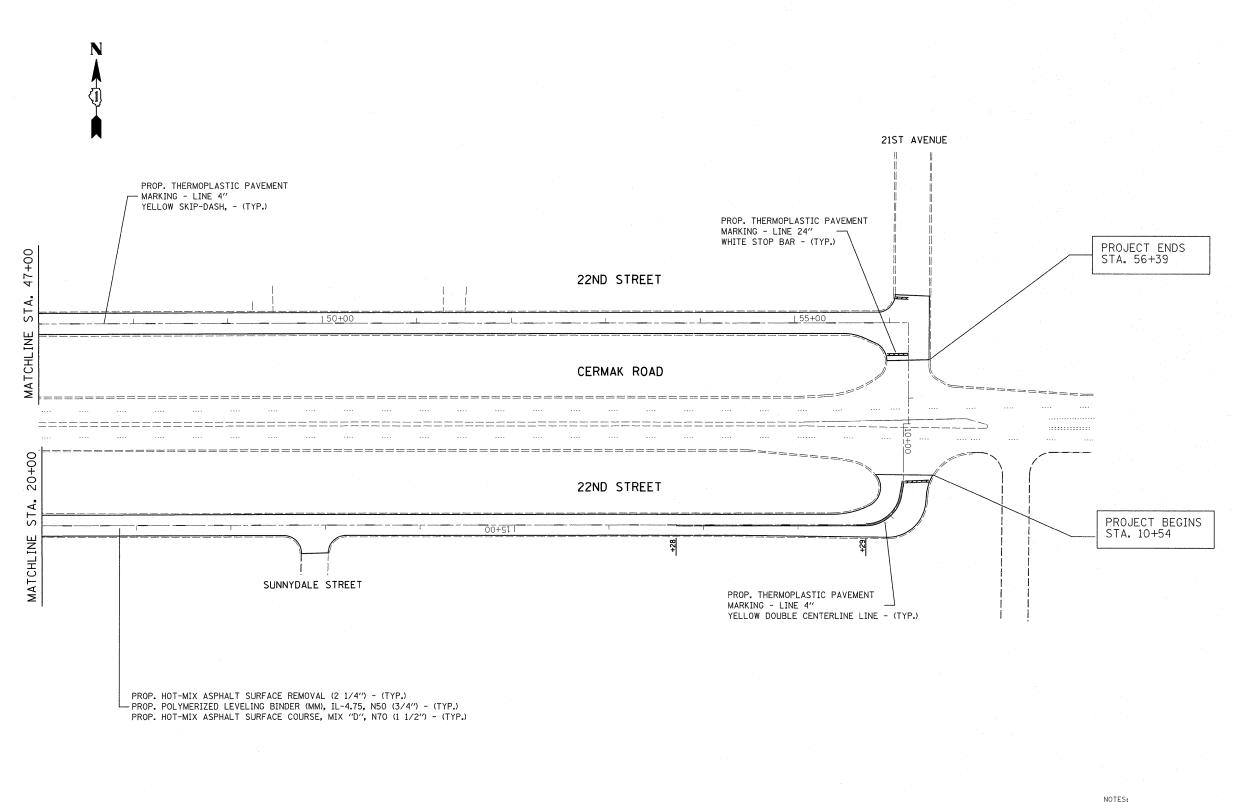
NOTES: LIMIT OF RESURFACING ON SIDE-STREETS THROUGH OUT THE IMPROVEMENT SHALL BE TO THE RADIUS OF RETURN OR AS DIRECTED BY THE ENGINEER.
