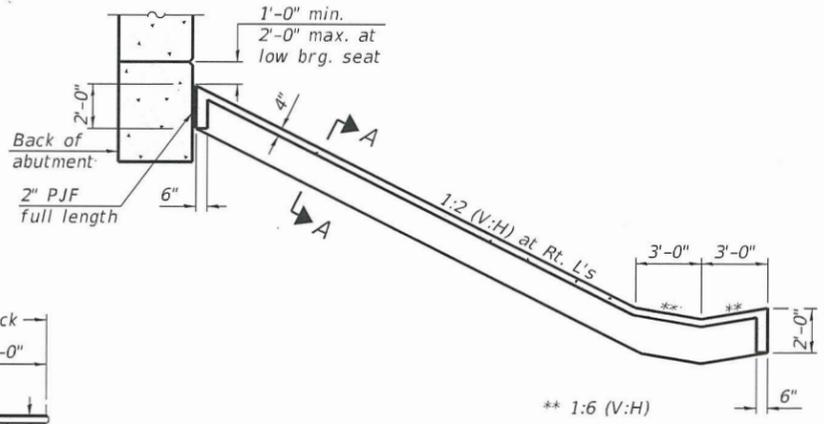
**SECTION THRU CONCRETE SLOPEWALL**
