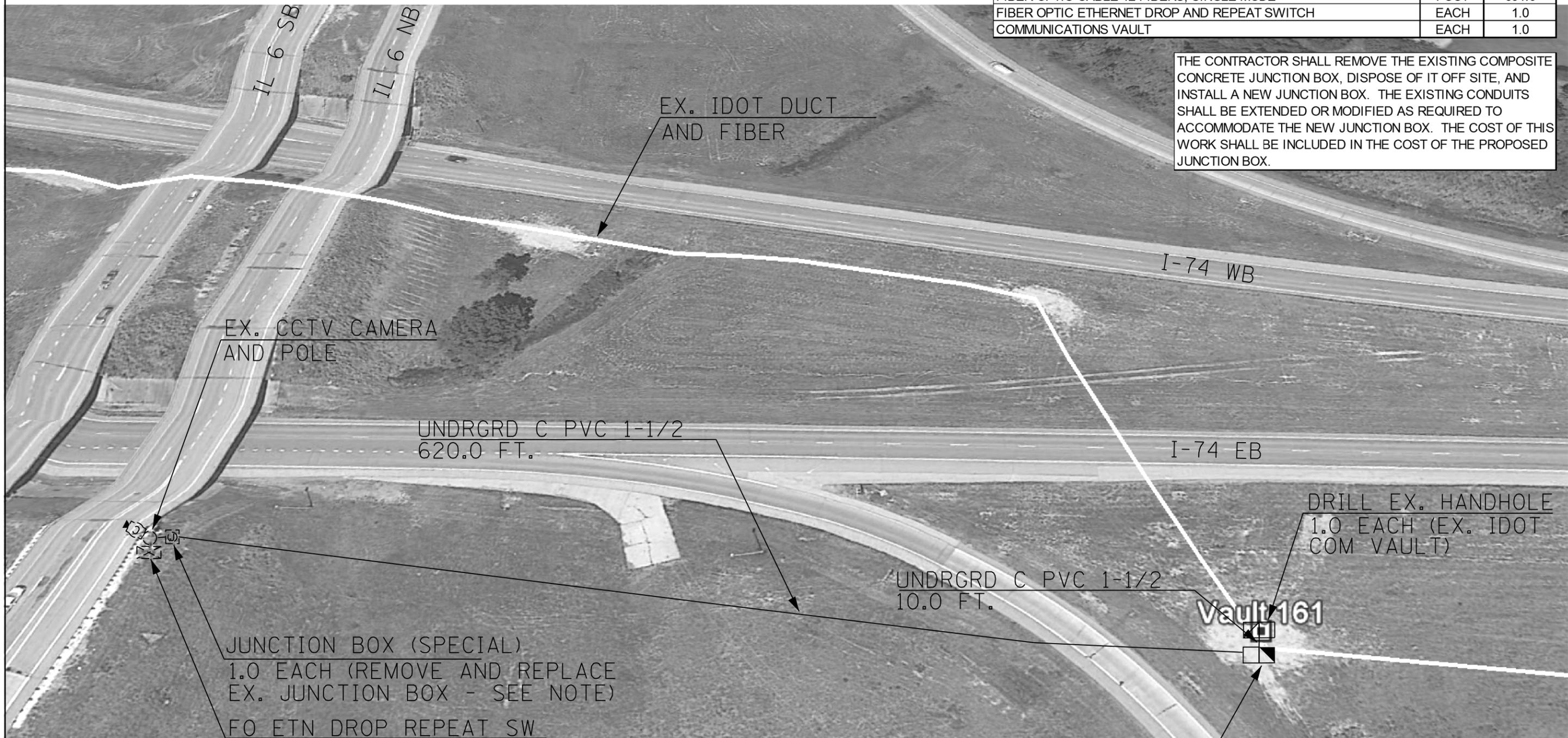
THE CONTRACTOR SHALL INSTALL 50 FT. OF SLACK FIBER IN THE PROPOSED COMMUNICATIONS VAULT
