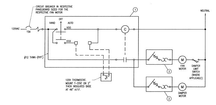
EXHAUST FAN CONTROL SCHEMATIC
