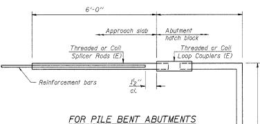
Bar Splicer for #5 bar Min. Capacity = 23.0 kips - tension Min. Pull-out Strength = 9.2 kips - tension No. Required =
