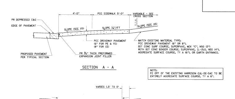
LEX/PR EDGE OF PAVEMENT PR COMBINATION CURB & GUTTER
