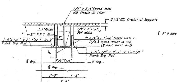
NOTE: Hatched area to be poured after beams are in place.
