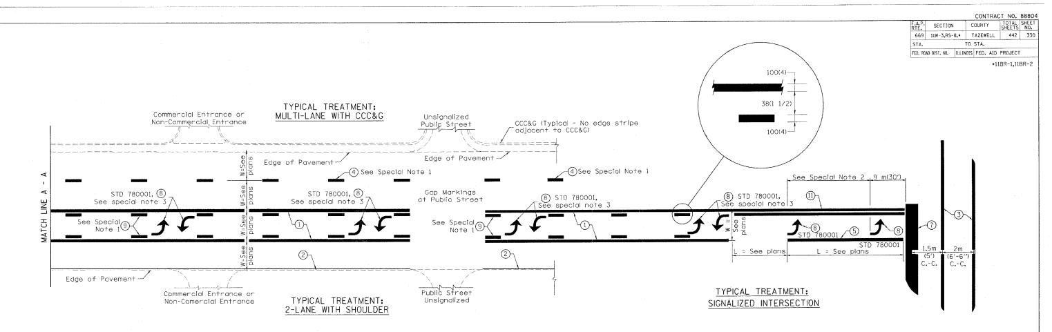
FLUSH PAVED MEDIAN: TWO-WAY LEFT TURN LANE WITH ONE-WAY LEFT TURN LANE AT SIGNALIZED INTERSECTION
