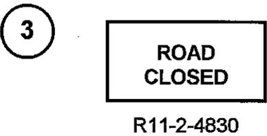
Mount on Type III Barricades as shown on Standard 702001 Detail for "ROAD CLOSED TO ALL TRAFFIC". Each Type III Barricade shall have two Type A Flashing Lights.
