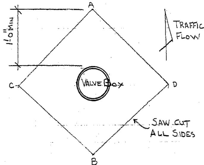
1. Water Valve box shall be adjusted after paving is completed.
