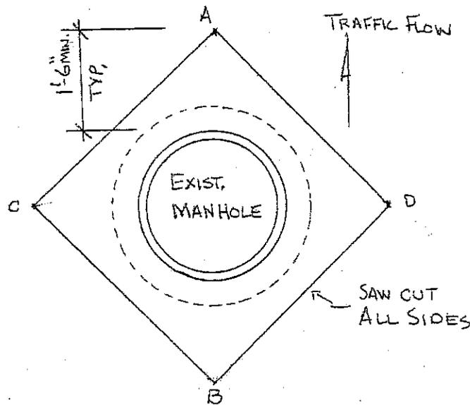
1. Adjust manhole after paving is completed.
