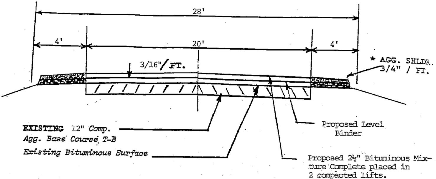
\* NOTE: Shoulders to be mowed by others prior to placement of aggregate.
