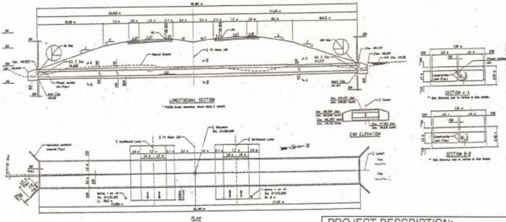
STATION 31+282 DOUBLE 12' X 5' X 302' BOX CULVERT
