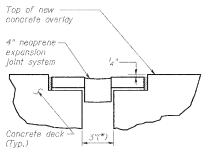
\* at 50°F. See Neaprene and Silicone Joint Schedule for required movement
